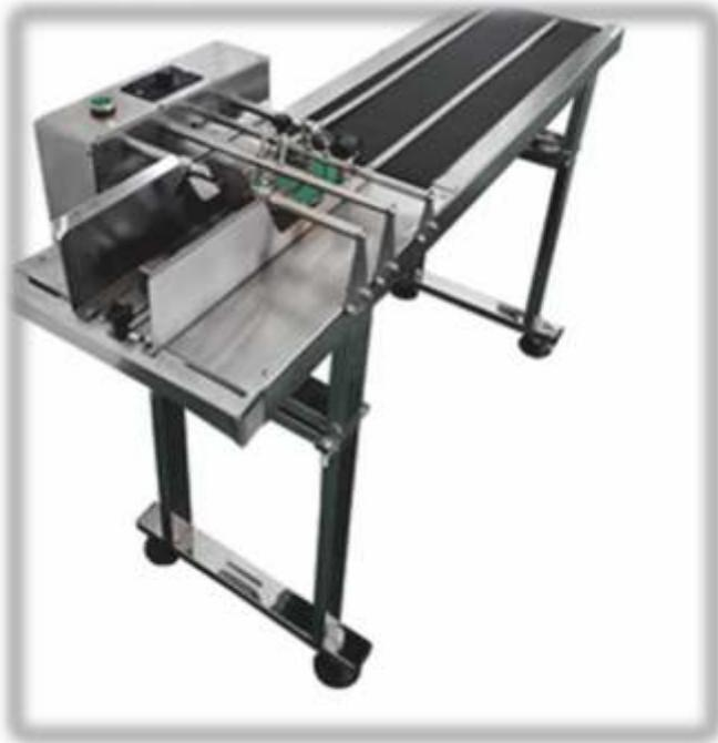
Friction feeders are ideally suited for the feeding separation and counting of flat products e.g. envelopes, phone cards, carton cuttings, inserts.
